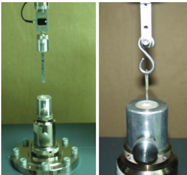
Fig 3. Specimen setup for testing the tensile bond strength in a universal testing machine.
