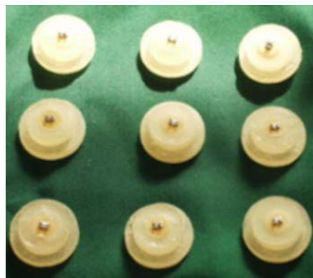
Fig 2. Specimens after mounting in acrylic resin.
