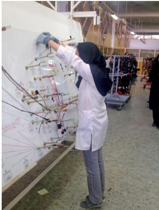
**Figure 2. Cable assembly unit (CABLE):** a worker is weaving wire standing on her tiptoes. The posture of her shoulders and upper arms is considerably deviated from neutral.
