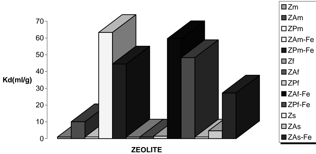
Fig. 2: Comparison of the natural (Zm, Zf, and Zs), synthetic (ZAm, ZPm, ZAf, ZPf, and ZAs) and modified zeolites (ZAm-Fe, ZPm-Fe, ZAf-Fe, ZPf-Fe, and ZAs-Fe)
