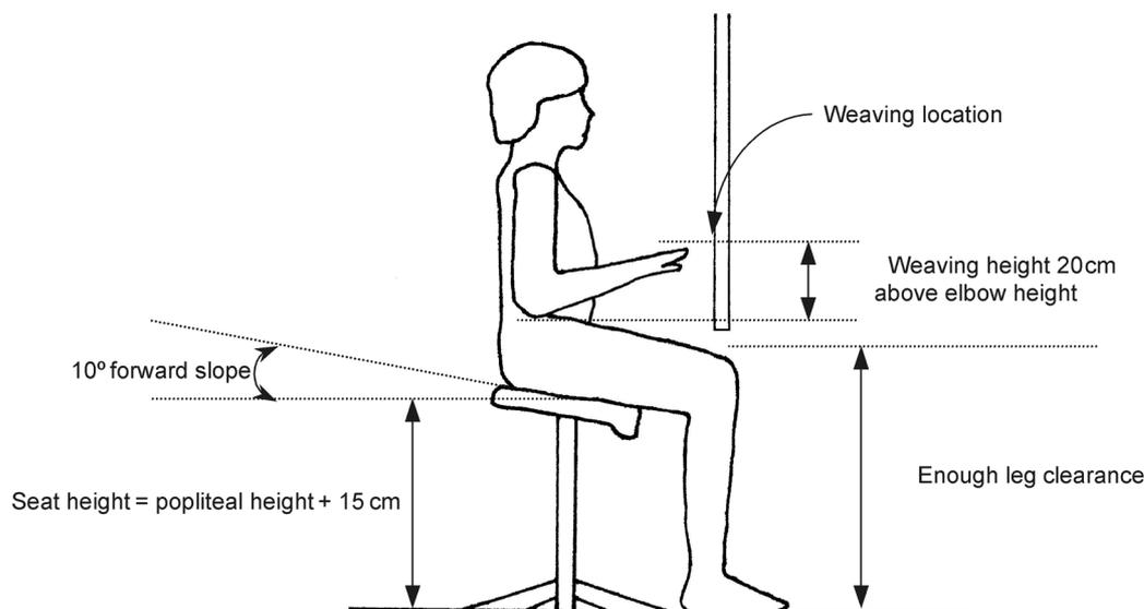
Figure 6. Guidelines for adjustment of a hand-weaving workstation.
