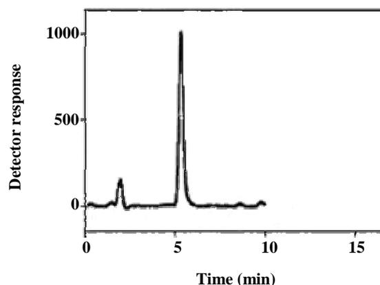
Fig. 2: Chromatogram of 1-OHP, mobile phase, 0.88% methanol/12% water; flow rate, 0.8 ml/min; analytical column, C<sub>18</sub> reversed phase; fluorescence detector at 242 and 388 nm; injection volume, 20  $\mu$ l; ambient air.
