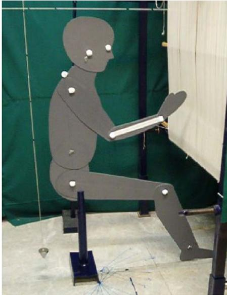
Fig. 6. The manikin used for determination of postural angle measurement accuracy. Markers are attached on the same landmarks as a real subject. Reference lines are visible in the picture.
