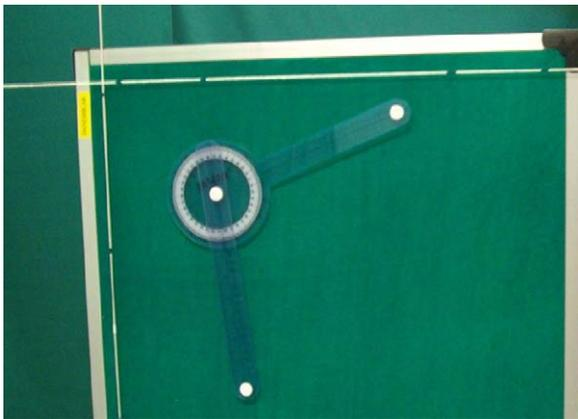
Fig. 5. Static test. Reflective markers attached to a standard goniometer.
