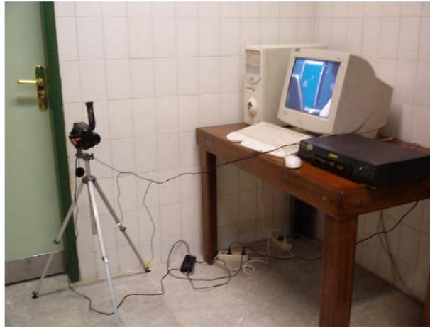
Fig. 1. The components of WEPAS. Video camera, video recorder, computer equipped with capture card and installed WEPAS software are parts of this system.
