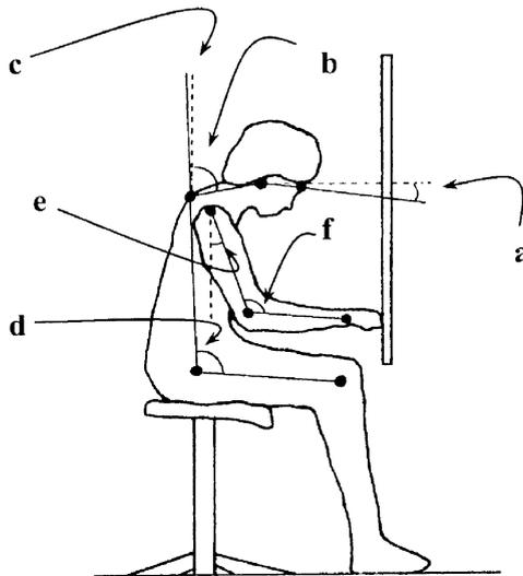
Fig. 3. Postural angles measured by WEPAS. Dotted lines are horizontal and vertical reference lines. a=HI, b=NI, c=TI, d=TA, e=AA and f=EA.
