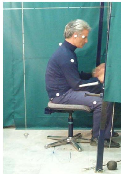
Fig. 2. A weaver is working in the experimental workstation. The horizontal and vertical reference lines (level and plumb lines, respectively) are seen in the picture. The reflective markers are attached on the anatomical landmarks including outer canthus, tragus, C7, greater trochanter, greater tubercle, lateral humeral epicondyle, styloid process of ulna and lateral femoral epicondyle.
