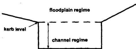
Figure 3. Definition sketch showing the hydraulic significance of the kerb level.
