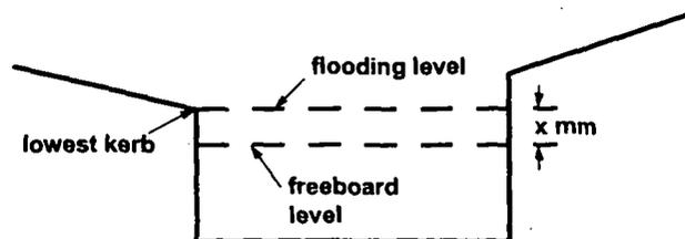
Figure 2. Definition sketch of flooding and  $x$  mm freeboard levels.
