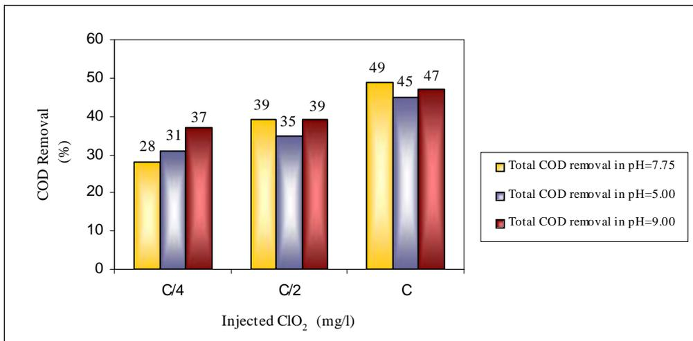
Figure 3: Total COD removal as a function of injected ClO<sub>2</sub> in various pH<sub>s</sub> of treatment
