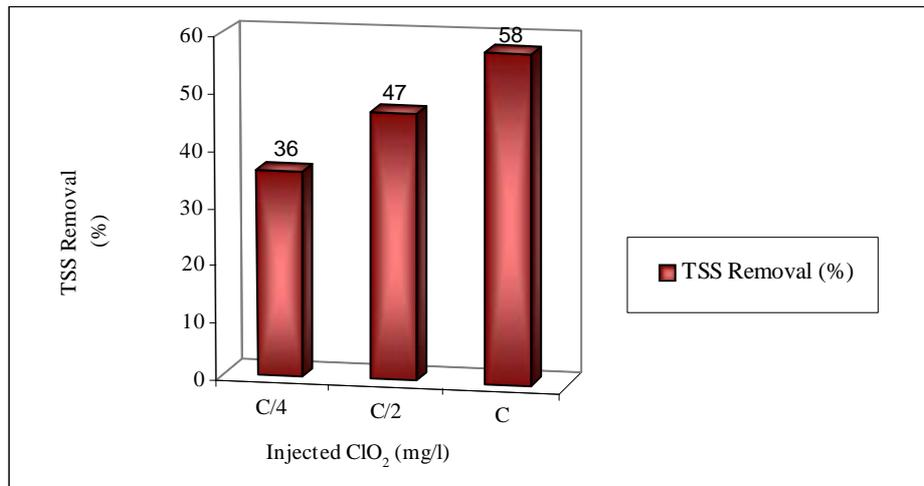
Figure 5: TSS removal as a function of injected  $\text{ClO}_2$  in contact time of 1 hour
