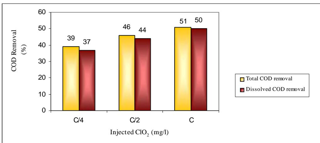
Figure 4: Total and dissolved COD removal as a function of injected ClO<sub>2</sub> in one hour contact time (C = influent COD concentration)
