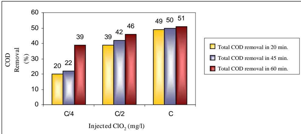
Figure 2: Total COD removal as a function of injected ClO<sub>2</sub> in different contact times (C= influent COD concentration)
