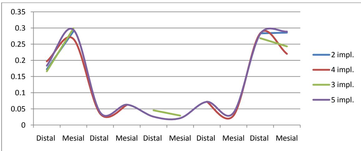
**Fig 4.** Von Mises stresses on cortical bone.
