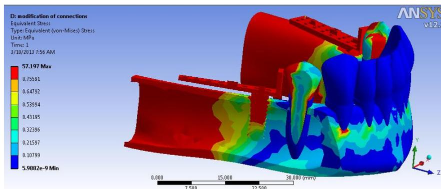
Fig 4. Stress contours when the implant was in the second premolar area.
