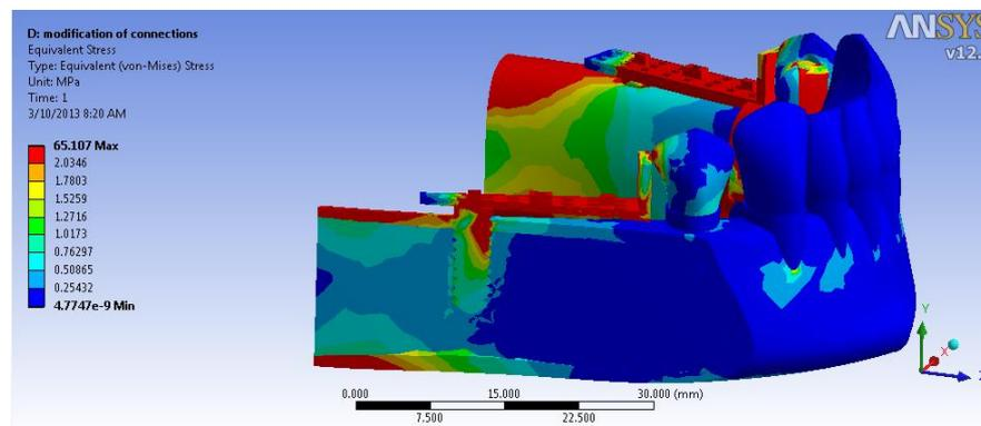
Fig 6. Stress contours when the implant was in the second molar location.
