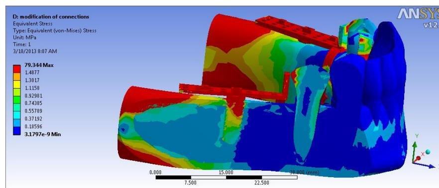
Fig 5. Stress contours when the implant was in the first molar area.
