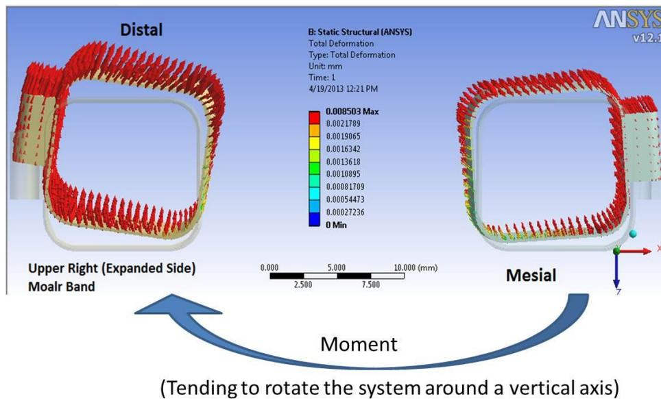
**Fig 5b.** The pattern of tooth movement shown in Figure 5a is viewed occlusally by tracing the band displacements. A distally driving force is shown to be combined with a yawing moment on molars.
