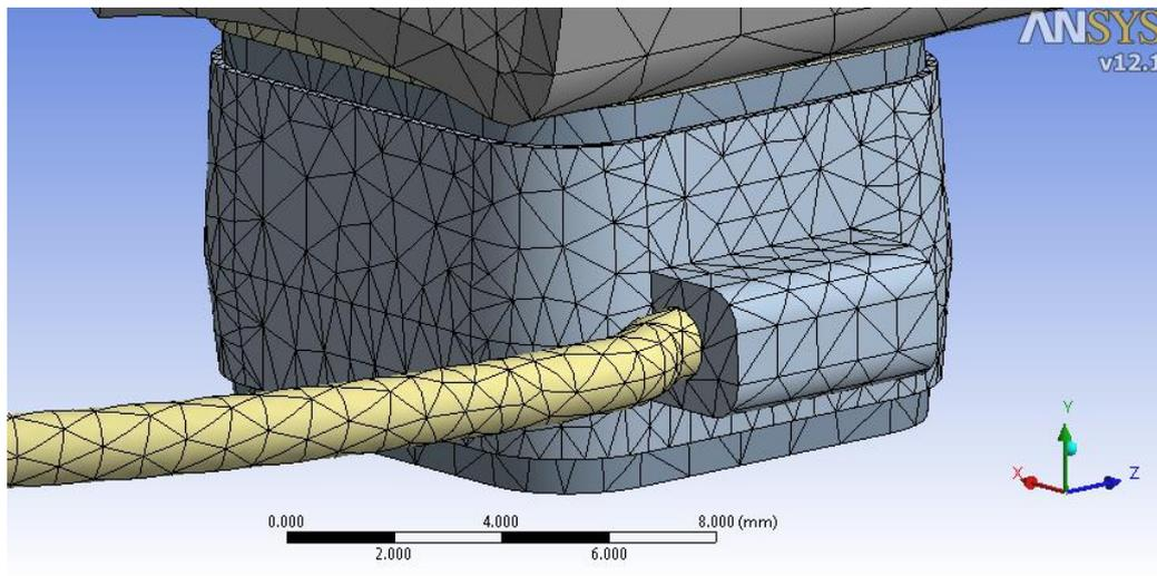
**Fig 1b.** Closer view of the 3D model showing the connection between the upper left molar, its band, and inner bow end.
