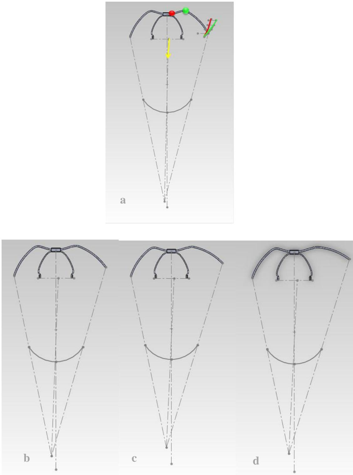
**Fig 2.** Four asymmetric headgear models produced by expansion of the outer bow. a) The green curve is selected for the outer bow expansion (with the green point as the center) which can produce a greater difference in the neck tangent line angles than the red curve with the red point as the center. The yellow vector shows the asymmetric force production. b, c, and d) Progressive steps of outer bow expansion.
