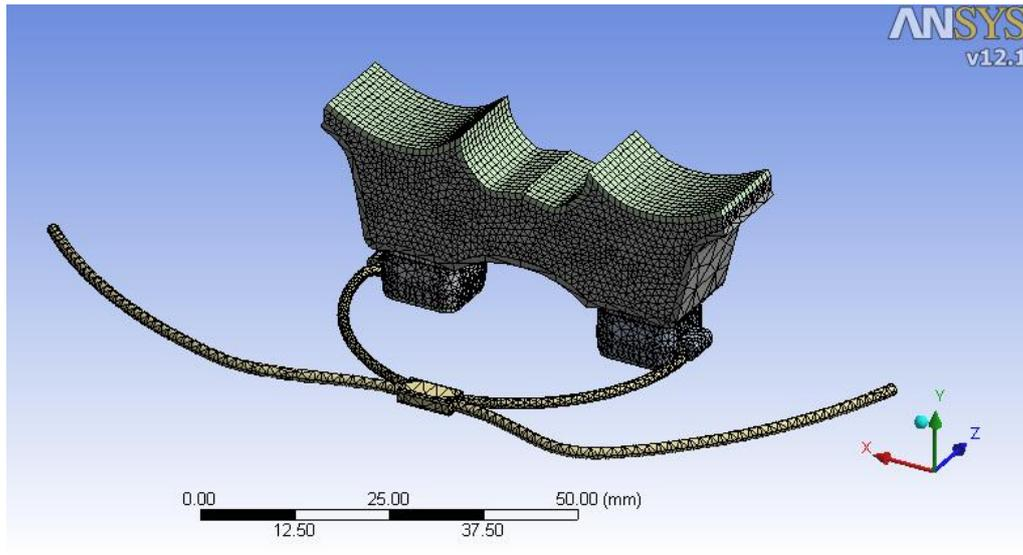
**Fig1a.** The meshed 3D model.
