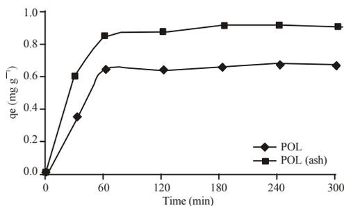
Fig. 1: Effect of contact time on the removal of Cd by POL and its ash (Adsorbent dosage = 2 mg l<sup>-1</sup> Cd concentration = 2 mg l<sup>-1</sup>)
