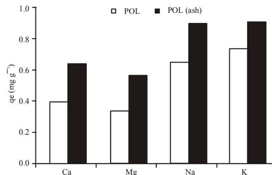
Fig. 4: The effect of light metals on adsorption capacity (Cd = 2 mg l<sup>-1</sup> and 2 mol l<sup>-1</sup> Ca, Mg, Na, K)
