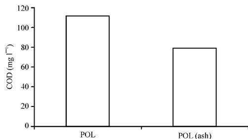
Fig. 8: The effect of 2 g l<sup>-1</sup> POL and its ash on increase COD (mg l<sup>-1</sup>) (120 min, pH=7, T= 24°C)
