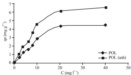
Fig. 3: Effect of Cd concentration on the removal of cadmium by POL and its ash (Adsorbent dosage = 2g l<sup>-1</sup> pH=7, T=24°C, 300 rpm, 120 min)
