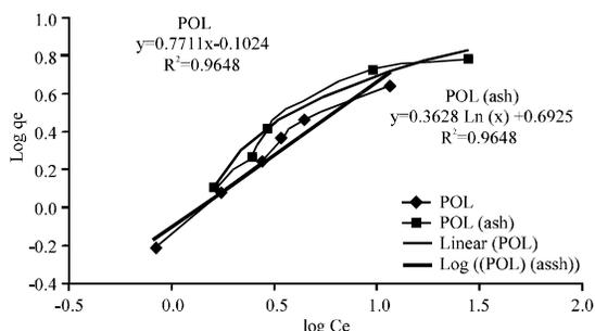
Fig. 7: The linearized Freundlich adsorption isotherm for Cd by POL and its ash
