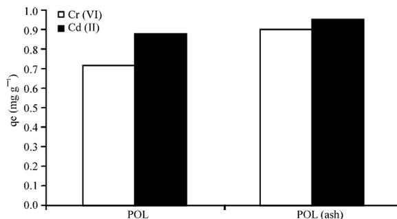
Fig. 5: Simultaneous adsorption of Cd (II) and Cr (VI) ions was studied, using a medium that contained 2 mg l<sup>-1</sup> of each metal ion
