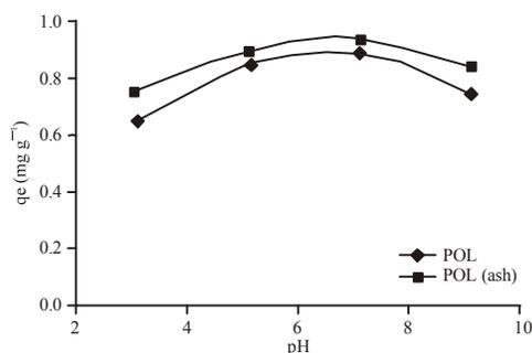
Fig. 2: Effect of pH on the removal of cadmium by POL and its ash (Adsorbent dosage = 2 g l<sup>-1</sup> Cd concentration = 2 mg l<sup>-1</sup>)
