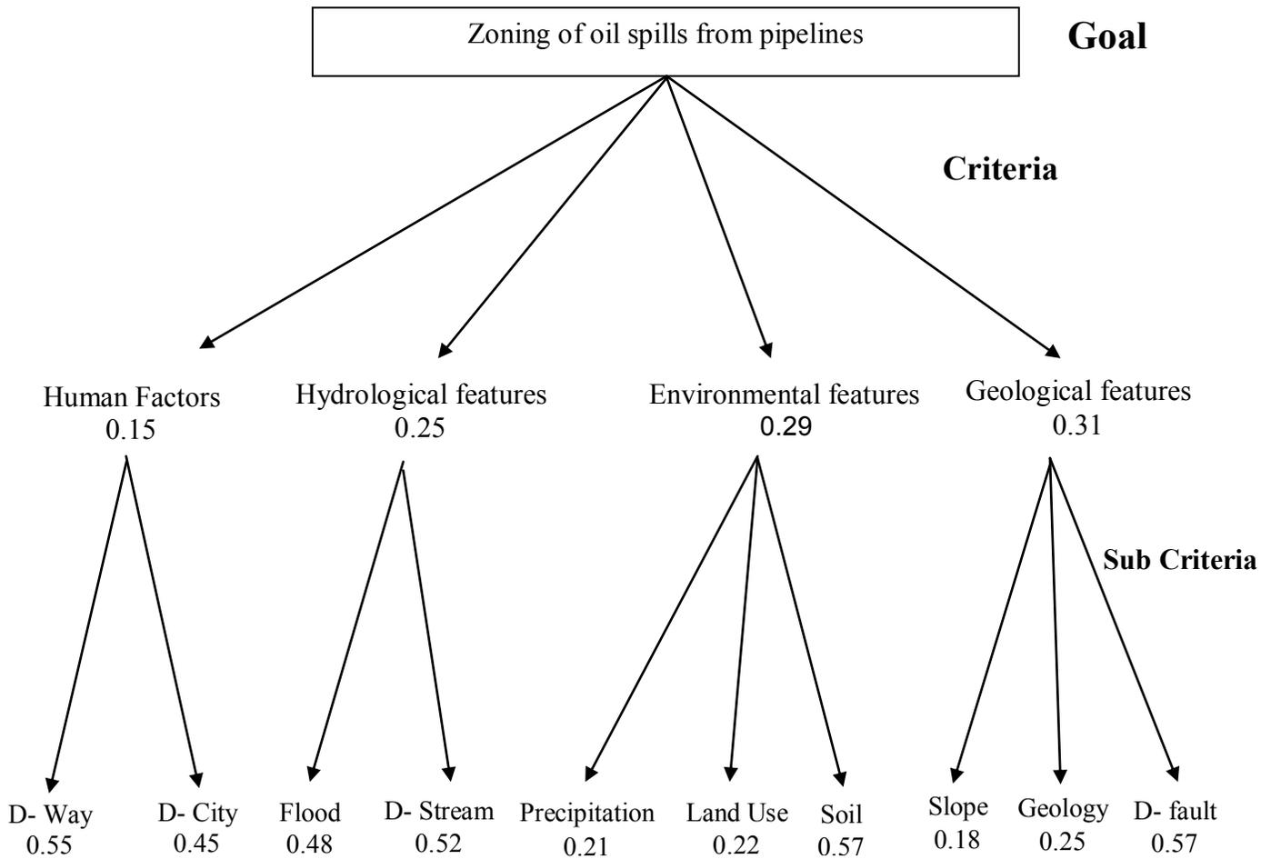
**Fig4.** Hierarchical structure of the zoning oil spills from pipelines
