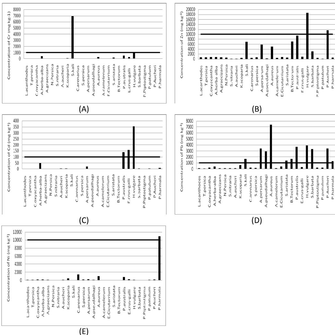
**Fig. 2.** Min of Metal Concentration of Cr (A), Zn (B), Cd (C), Pb (D) and Ni (E) in plants (shoots + roots) collected from raw sewage polluted area of Eshthard industrial park (three replicates).
