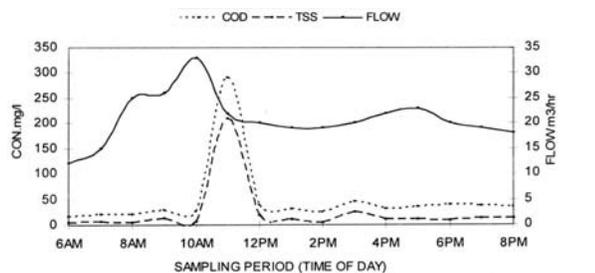
Fig. 4. Variation of COD and Soluble COD in effluent Within sampling period
