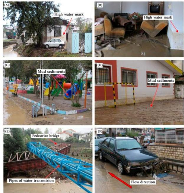
Fig. 6. Observations following the flood event: (A) Wall collapse and flood flow to a house at (P1), (B) Inundated first floor and home appliance and furniture damages at (P2), (C) Flood has passed through the playground, (D) Flood has affected the school yard at (P3), (E) Damaged urban infrastructure at (P4), and (F) Flood has carried cars at (P5).
