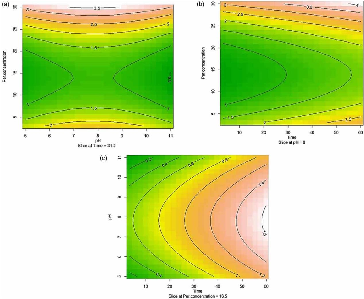
**Figure 2** | Contour plot of log inactivation of *Bacillus subtilis* spores by a combined UV/persulfate process. Shows the effect of (a) persulfate concentration and pH, (b) persulfate concentration and contact time, (c) pH and contact time, and their mutual interactions on *B. subtilis* spore inactivation.
