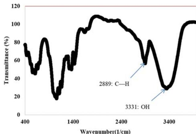
Fig. 3. FTIR spectrum of cotton-graphene oxide adsorbent.
