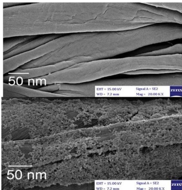
Fig. 2. FE-SEM images of cotton and cotton-graphene oxide.
